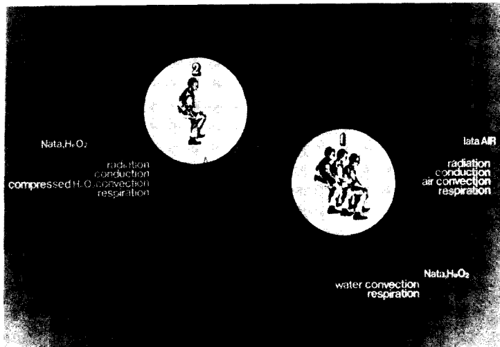
Fig. 1. Thermal environments associated with lockout submersibles, showing major heat transfer avenues for each environment.
