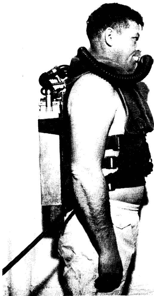
FIG. 4. Prototype of deep dive mixed gas breathing apparatus used at the U. S. Navy Experimental Diving Unit.
