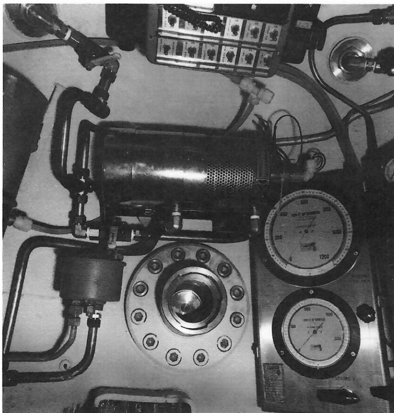
Fig. 10.8. Hot-water-supplied heat-exchanger with electric blower for heating diving bell (by Kinergetics Inc.).
