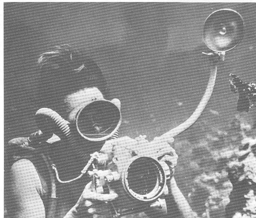
Fig. 74. Diver-lensman using oxygen rebreather lung and the Franke and Heidecke Rolleimarin camera housing with flash attachment. (Burleigh Brooks Photo)
