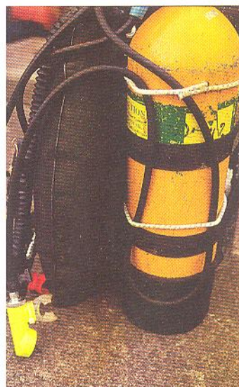
Two metre hose retained by inner tube.
